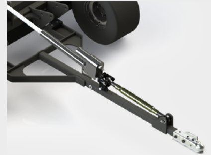
6. ADJUSTABLE HITCH ACCOMMODATES VARIOUS TOW VEHICLES FOR PRECISE FIELD LEVELLING
